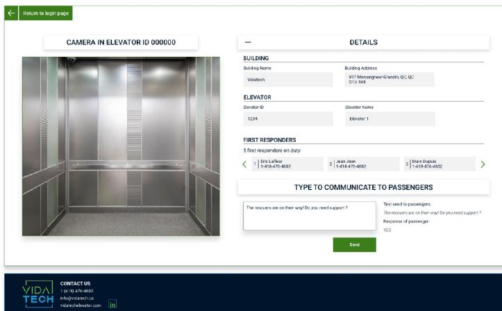
5 **Prioritize audio communication via the handset.** If the passenger is unable to communicate vocally, use the chat area to send messages on the elevator screen.
