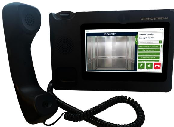
3 To end the conversation. Press the red button at the bottom of the screen.
